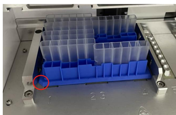
Figure 4. Put the single kit docking into the instrument
