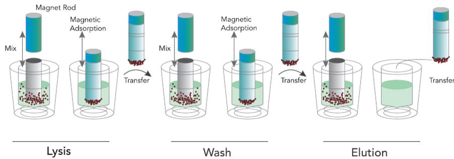
Figure 1. Schematic Diagram of Panall 8000 MD System
