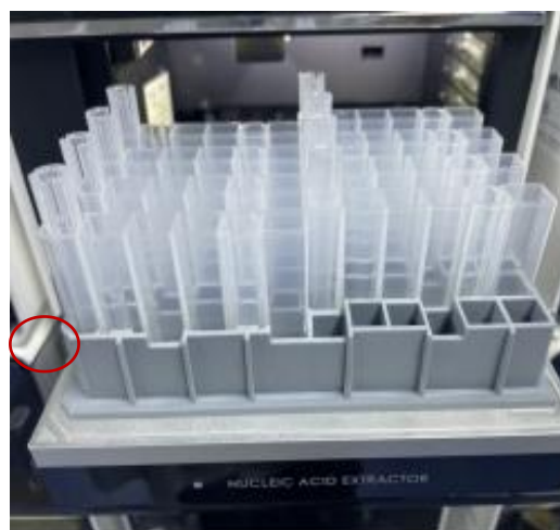
Figure 5. Put the single kit docking into the instrument
