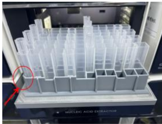
Figure 5. Put the single kit docking into the instrument
