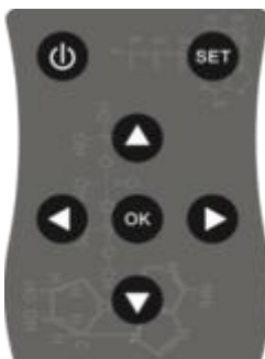
Fig 2.2 Biolum detector keyboard
