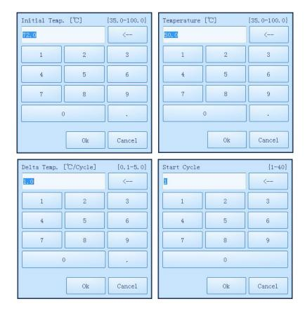
Figure E-3.4a. Step Edit Window - Touchdown Step Parameter Setting
