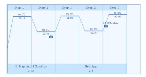
Figure E-4.4. Run Monitoring Diagram - Temperature Program
