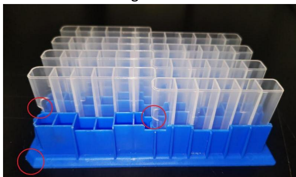
Figure 2. Put the 6 strip tube on the single kit docking
