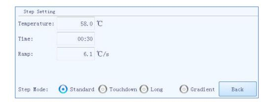
Figure E-3.3. Temperature Setting Sub-tab - Step Edit Window - Standard Step Mode
