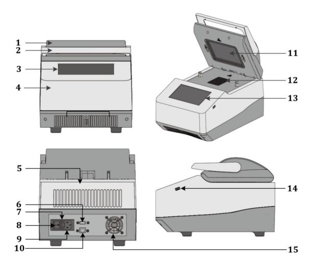
Figure A-1. Gentier Instrument Structure
