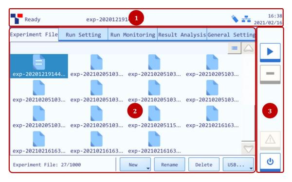
Figure E-1. Instrument Software Main Interface
