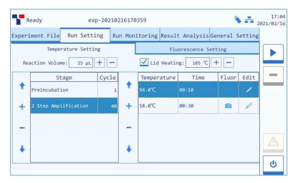
Figure E-3. Run Setting Interface - Temperature Setting Sub-Tab
