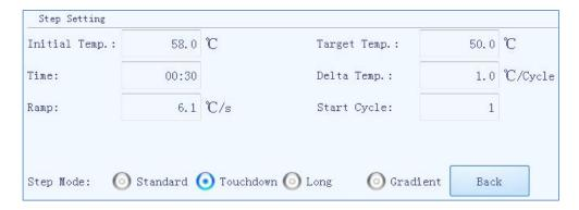
Figure E-3.4. Temperature Setting Sub-tab - Step Edit Window - Touchdown Step Mode
