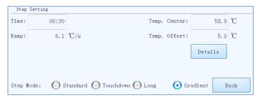
Figure E-3.6. Temperature Setting Sub-tab - Step Edit Window - Gradient Step Mode
