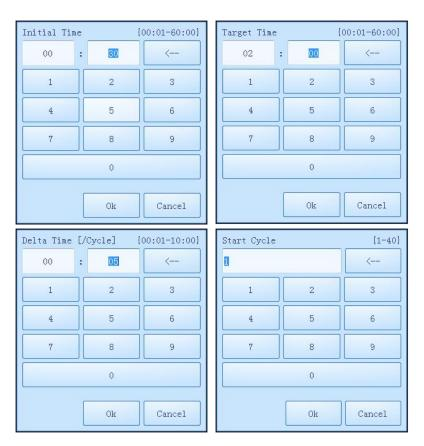
Figure E-3.5a. Step Edit Window - Long Step Parameter Setting
