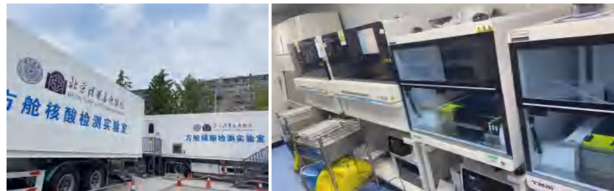
Beijing Tsinghua Changgeng Hospital Landing container mobile laboratory (two cabins). Daily testing capability can be up to 10,000 tubes per day in each cabin.
