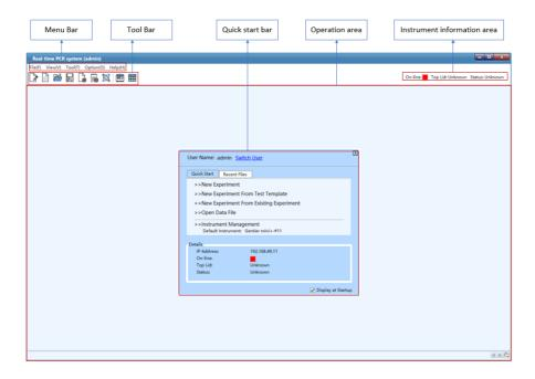
Figure E-1.2 Startup Interface of Application Software
