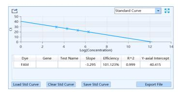
Figure E-10.2 Abs Quant Analysis Interface - Standard Curve Functional Module
