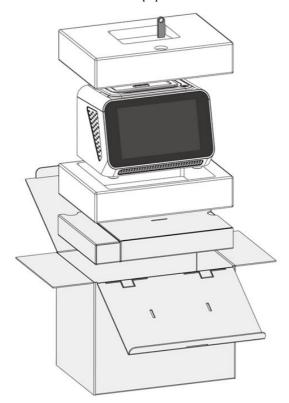
Figure B-1. Exploded View of Package
