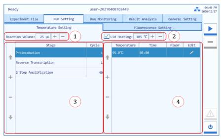
Figure F-2.2a Experiment File Tab – Temperature Setting Sub-tab
