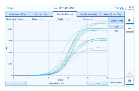
Figure F-3.1 Run Monitoring Diagram - Real-time Amplification Curve
