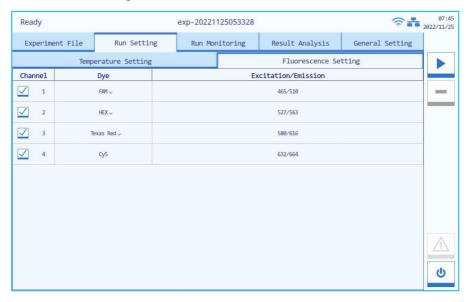
Figure F-2.3. Run Setting Interface - Fluorescence Setting Sub-tab
