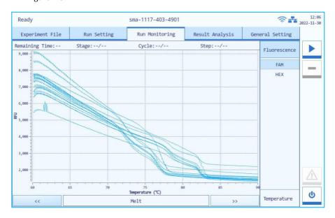
Figure F-3.2 Run Monitoring Diagram - Real-time Melting Curve
